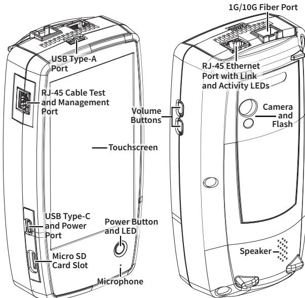
The LinkRunner® 10G is a rugged, hand-held tool for testing and analyzing wired copper and fiber Ethernet networks. This Multi-Gig Network Tester features applications developed by NetAlly for wired network measurement and validation.
